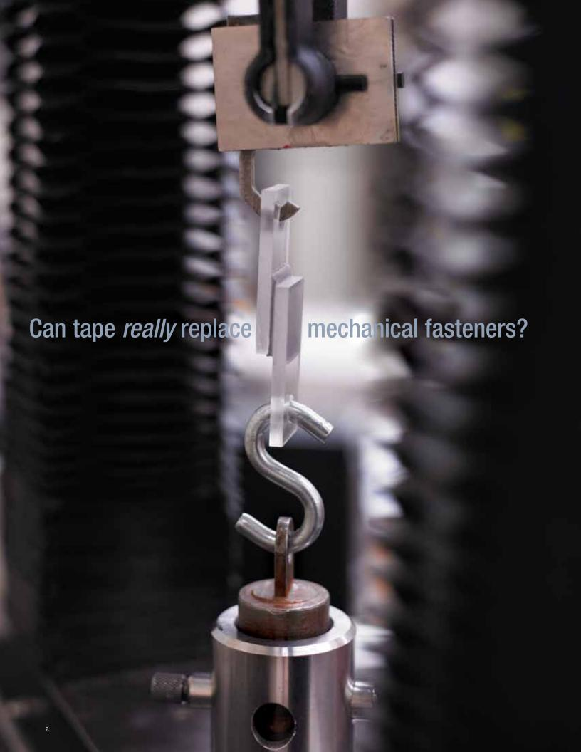
Yes. Acrylic foam tape is a specialty bonding tape that is a proven high-strength alternative to screws, rivets, welds and other forms of mechanical fasteners. While a screw or a rivet can join two substrates at a single point, specialty bonding tape permanently adheres one substrate to another and spreads the stress load across the entire length of the joint. Once substrates are joined with high-strength bonding tape, a virtually indestructible "weld" is created.
